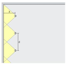
For good longitudinal uniformity, the luminaire spacing (d) of Parscan wallwashers may be up to 1.5 times the distance to the wall (a).
