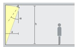
Wallwashing For uniform vertical illuminance, the distance (a) of Parscan lens wallwashers from the wall should be around one third of the room height (h). This results in an angle of tilt ( $\alpha$ ) of approx. 35°.
