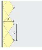
Wide luminaire spacing with wallwashing With ERCO's advanced lighting technology, Iku luminaires can be installed at up to 1.5 times the wall spacing, providing excellent light distribution.
