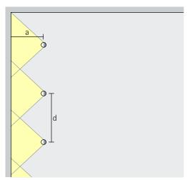
For good longitudinal uniformity, the spacing (d) of Eclipse 48V lens wallwashers can be up to 1.5 times the distance to the wall (a).
