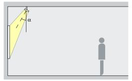
Accentuation Works of art, merchandise and architectural details are effectively accentuated with Parscan. The ideal angle of tilt ( $\alpha$ ) for this is around 30°. The object is modelled without distorting the effect as a result of excessive shadowing. It also prevents shadows cast by the observer.
