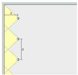
For good longitudinal uniformity, the luminaire spacing (d) of Optec wallwashers may be up to 1.5 times the distance to the wall (a).
