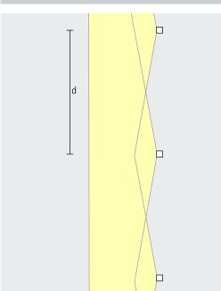
The spacing between two luminaires may be up to 2m. The luminaires may be spaced apart even further for visual guidance.
