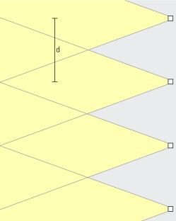
The spacing between two luminaires may be up to 2m. The luminaires may be spaced apart even further for visual guidance.
