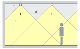
**General lighting**For the uniform illumination of office workplaces, the luminaire spacing (d) between two Jilly downlights may be up to 1.5 times the height (h) of the luminaire above the working plane (rough guide).
