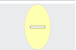
Jilly linear, with oval wide flood distribution of light transverse to the luminaire, orients itself to luminaire alignment as highly proven for office applications.
