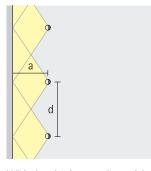
Wide luminaire spacing with wallwashing With ERCO's advanced lighting technology, Iku luminaires can be installed at up to 1.5 times the wall spacing, providing excellent light distribution.
