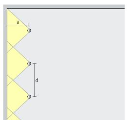
For good longitudinal uniformity, the spacing (d) of Eclipse lens wallwashers may be up to 1.2 times the distance to the wall (a).
