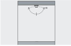
**Display case lighting** Semi-recessed luminaires are particularly discreet and can be installed in the showcase ceiling and floor. Mounting frames for one, two or four light heads are optionally available.
