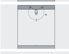
Display case lighting Surface-mounted luminaires are perfect for illuminating exhibits from different directions. The swivel range of  $(\alpha)$  270° is directed away from the mounting surface. Mounted on the showcase ceiling, their light is directed downwards – from the showcase floor, however, they illuminate upwards. The light heads can be infinitely rotated in a circle.
