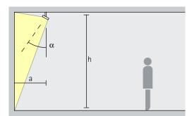
Wallwashing For uniform vertical lighting, the distance to the wall (a) of Parscan wallwashers should be around one third of the room height (h). This results in an angle of tilt ( $\alpha$ ) of approx. 35°.
