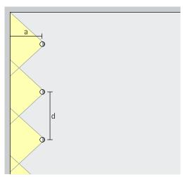
For good longitudinal uniformity, the luminaire spacing (d) of Parscan wallwashers may be up to 1.2 times the distance to the wall (a).
