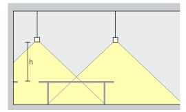
**General lighting**To achieve a high level of uniformity and good facial recognition when illuminating single workstations, Jilly pendant luminaires with oval wide flood light distribution should be suspended to the left and right of the desk at a height (h) of approx. 1.2m above the desk plane.
