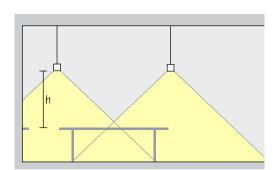
**General lighting**To achieve a high level of uniformity and good facial recognition when illuminating single workstations, Jilly pendant luminaires with oval wide flood light distribution should be suspended to the left and right of the desk at a height (h) of approx. 1.2m above the desk
