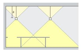
Indirect lighting on bright ceilings increases the visual comfort due to diffusely reflected light. The room also appears to be higher. The luminaire should be suspended from a height of at least 0.5m.
