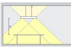
**General lighting**To achieve a high level of uniformity and good facial recognition when illuminating single workstations, Jilly pendant luminaires with extra wide flood light distribution should be suspended at a height (h) of approx. 1.2m above the desk
