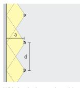
Wide luminaire spacing with wallwashing Efficient ERCO photometrics allow certain luminaires to be spaced unusually far apart at up to 1.5 times the distance to wall.
