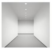
**Double wallwasher** The special light distribution of the double wallwashers efficiently illuminates the opposite walls of corridors. The diffuse, reflected light from the walls also illuminates the floor and ceiling.
