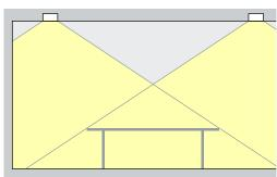
**General lighting**For efficient workplace illumination in the office, with optimal uniformity and good facial recognition, the luminaire spacing (d) of Compar downlights with oval wide flood distribution (d) may be up to 1.5 times the height (h) of the luminaire above the working plane.
