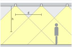
**Linear lighting**As a rough guide for uniform illumination, the luminaire spacing (d) between two Compar downlights installed in a row may be up to 1.5 times the height (h) of the luminaire above the working plane.
