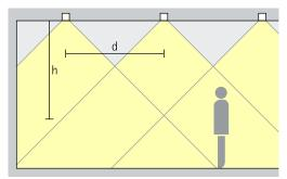
**General lighting**For optimum general lighting, the luminaire spacing (d) between two Compar downlights may, as a rough guide, be up to 1.5 times the height (h) of the luminaire above the working plane.
