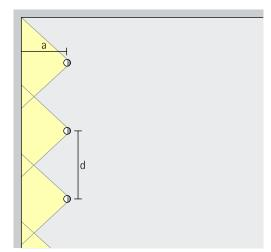
For good longitudinal uniformity, the spacing (d) of Compar lens wallwashers may be up to 1.3 times the offset from the wall (a).
