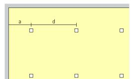
The wall offset should be half the luminaire spacing.
